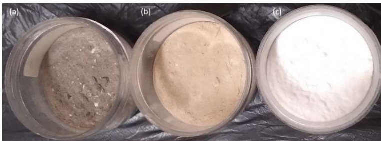
Fig.-2: Biosilica Washed with 20% HCl on the Baking of (a) 200, (b) 400, and (c) 600°C
