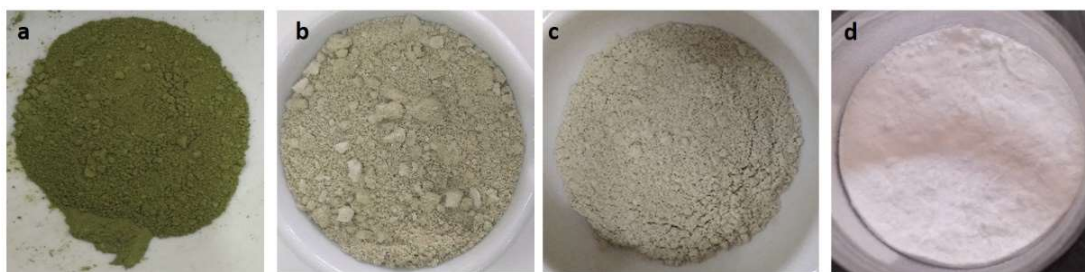
Fig.-3: Samples (a) biomass of Navicula sp. TAD, (b) Frustule Waste, (c) 20% HCl Washed Frustule Waste, (d) Biosilica of Frustules Waste After Baking
