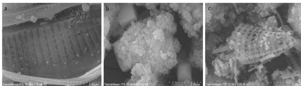
Fig.-4: SEM Images of (a) Untreated Diatom Biomass, (b) Waste Frustule, (c) Biosilica of Frustule Washed with 20% HCL Baked at 600 °C
