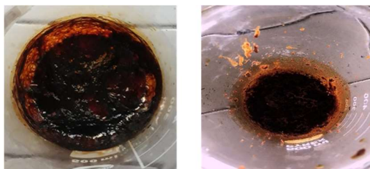
Fig.-1: Results of Microwave Heating (a) Molasses Without a Passivation Agent (b) Molasses with the Addition of a Passivation Agent
