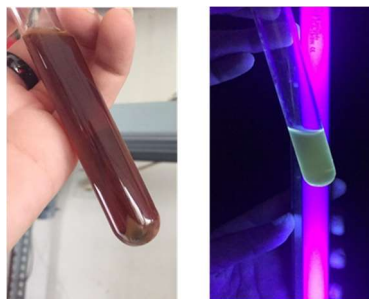
Fig.-4: Carbon Dots Solution with Passivation Agent (a) in Visible Light (b) in UV Light
