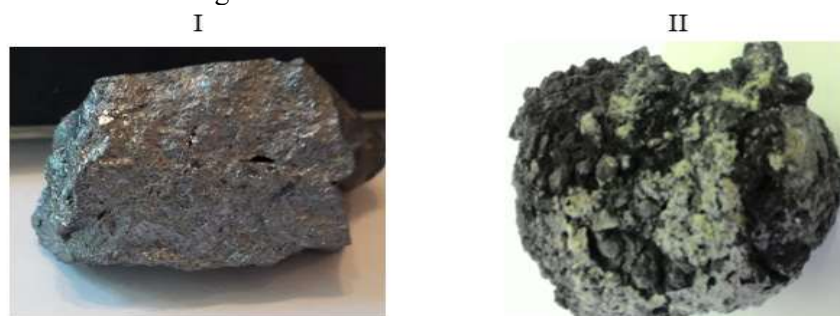
I – ferroalloy, II – calcium carbide Fig.-7: Products of Chilisai phosphorite smelting
