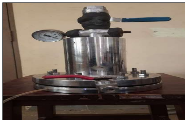
Fig.-4: Dead-End Filtration Setup
