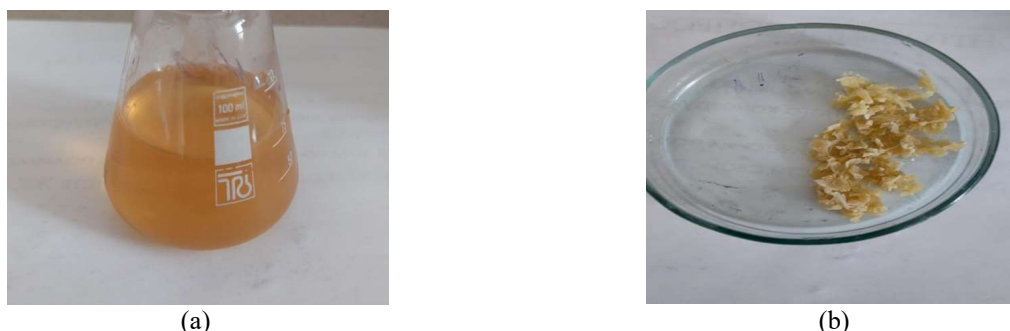
Fig.-3: (a) Copolymer Based on Acrylonitrile and Vinyl Sulfonic Acid; (b) Dried Polymer
