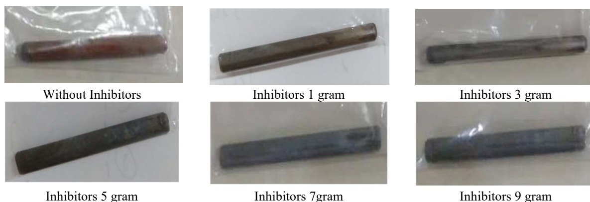
Fig.-4: Iron Plate After Soaking Without Inhibitor and Adding Inhibitor Purple Sweet Potato Leaf Extract with Soaking Time of 12 day
