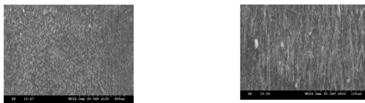
Fig.-6(a): EuBz-ap - PU(100:60) Before and After immersion in 3.5% NaCl
