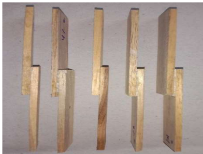
Fig.-2: Prepared Wood Block Samples for Moisture Resistance Testing
