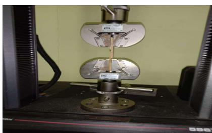
Fig.-3: Determination of Tensile Strength of Na 2 SiO 3 Adhesive on Wood Blocks
