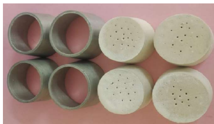
Fig.-1: Setting Time Moulds and Blocks of MOC
