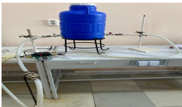
Fig.-2: Installation Diagram for Obtaining Films on the Surface of a Steel Sample
