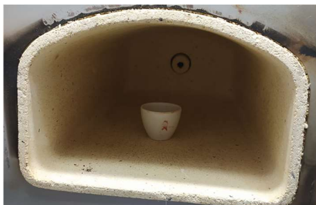
Fig.-4: Muffle Furnace
