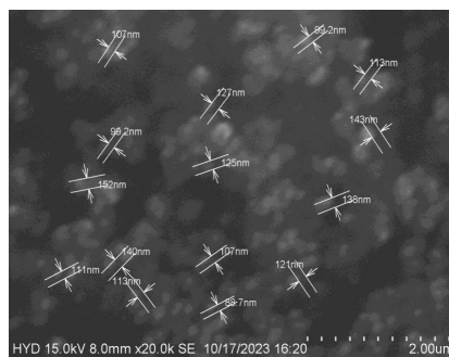
Fig.-6: SEM Analysis of MTS-Cu NPs
