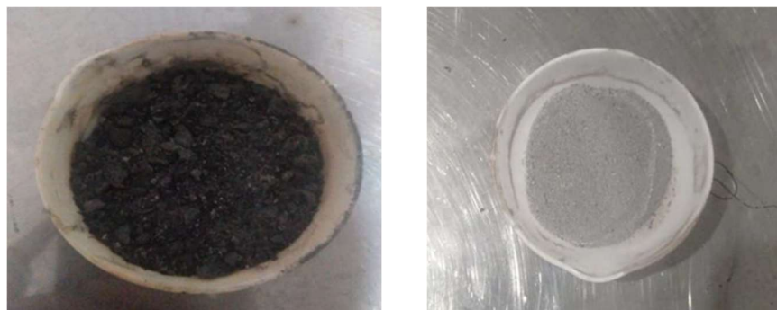
Fig.-1: Boiler Scale Ash and Boiler Scale Ash after Furnace
