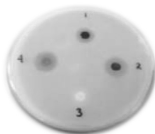
Fig.-2: The Result of The Antifouling: N -Hexane (1), Ethyl Acetate (2), Acetone (3) Extracts, and Positive Control (4)
