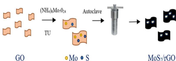
Fig.-2: Synthesize of the \text{MoS}_2 Doped rGO
