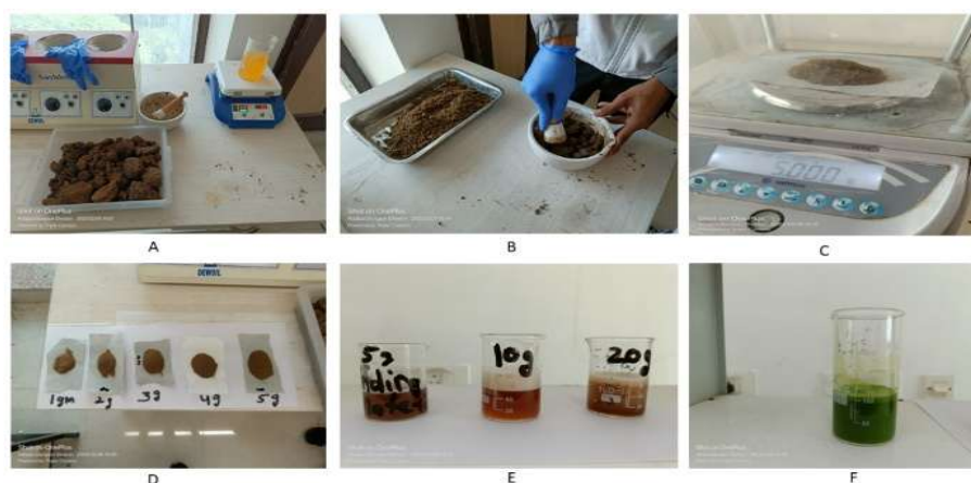
Fig.-2: Process of Cow Dung Paint Production: (A-C) Preparation (Weighing, Crushing and Mixing) of Raw Materials (Cow Dung, Cow Urine); (D) Cow Dung Powder in Different Amounts (E) Preparation of Binding Material Using Moringa Tree Leaves (F) Azadirachta indica Tree Leaves Extract (Pest Repellent)
