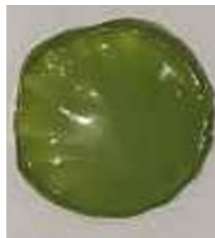
Fig.-2: Membrane Prepared for Barium Selective Electrodes
