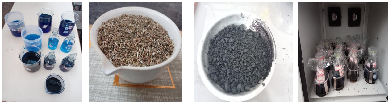
Fig.-2: Shows (a) Vat Dye Prepared for Analysis, (b) Raw Parthenium Powder, (c) Activated Powder, (d) Agitation
