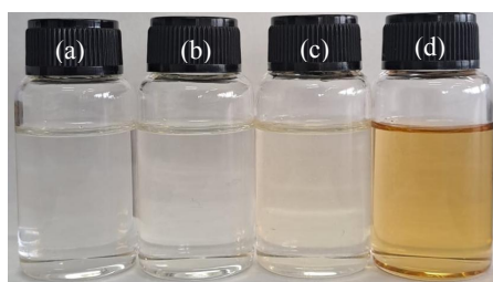
Fig.-1: Visual Characteristics of Synthesized Choline Chloride–Based Natural Deep Eutectic Solvents (NADES) with different Hydrogen Bond Donors and Molar Ratios: (a) ChCl–Glu (1:2, 20% water), (b) ChCl–Fr (1:2, 20% water), (c) ChCl–Mal (1:1, 20% water), and (d) ChCl–Xyl (1:1, 30% water)
