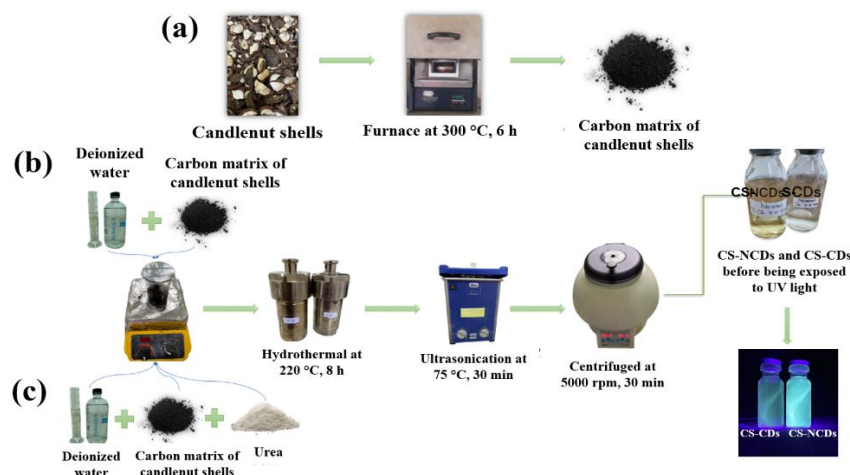
Fig.-1: Schematic Representation of (a) the Carbonisation of CS, (b) the Fabrication of CS-CDs, and (c) the Preparation of CS-NCDs via the Hydrothermal Synthesis
