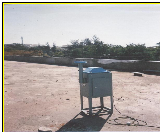
Plate-2: Respirable Dust Sample at Hingna Site
